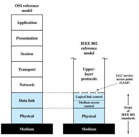
Figure 15.5 IEEE 802 Protocol Layers Compared to OSI Model
