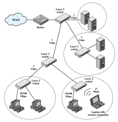
Figure 15.14 Typical Premises Network Configuration
