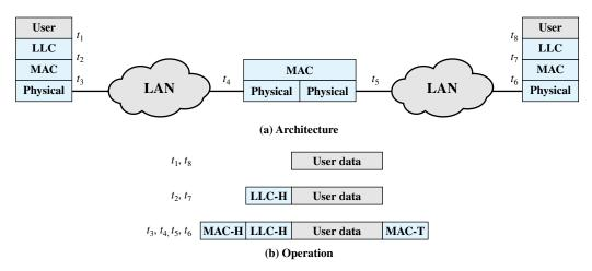
Figure 15.9 Connection of Two LANs by a Bridge
