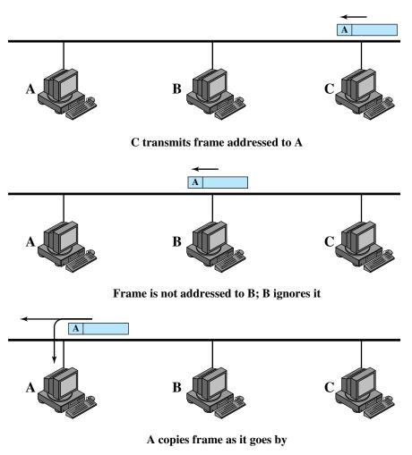
Figure 15.3 Frame Transmission on a Bus LAN
