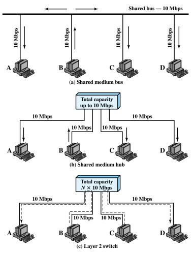
Figure 15.13 Lan Hubs and Switches
