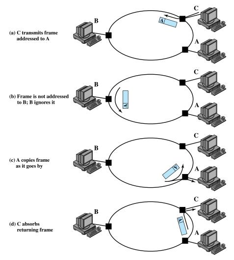
Figure 15.4 Frame Transmission on a Ring LAN
