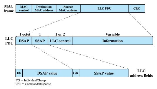
Figure 15.7 LLC PDU in a Generic MAC Frame Format
